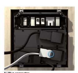
**5 | Plug connector**Self-locking and coded plug connectors facilitate faultless mounting with the device cup. To release, unlatch the grey spring catch with a turn screw.
